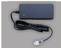
external power supply
